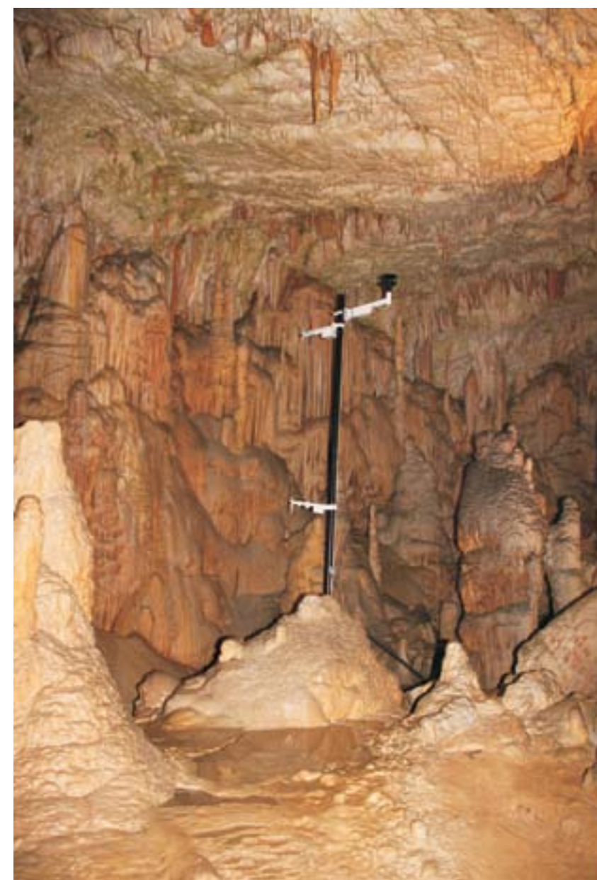
Fig. 3: Climatic monitoring in the Lepe jame, meteorological station (photo: Stanka Šebela).
