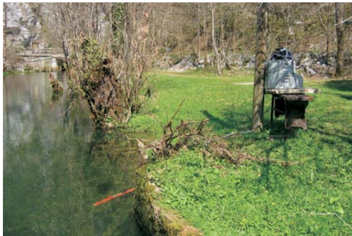
Fig. 3: An automatic sampler was set up at the Bilpa spring to collect samples.
