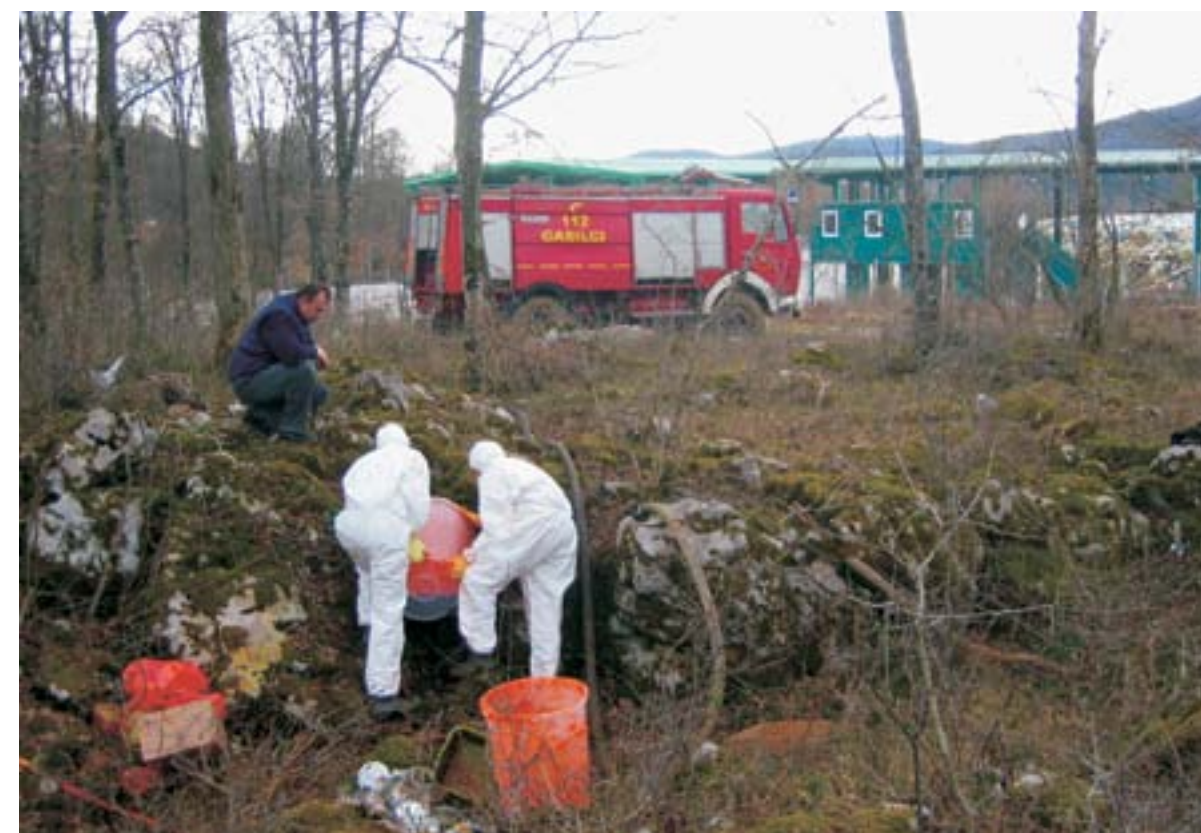
Fig. 2: Injection of uranine on the edge of the Mozelj landfill.
