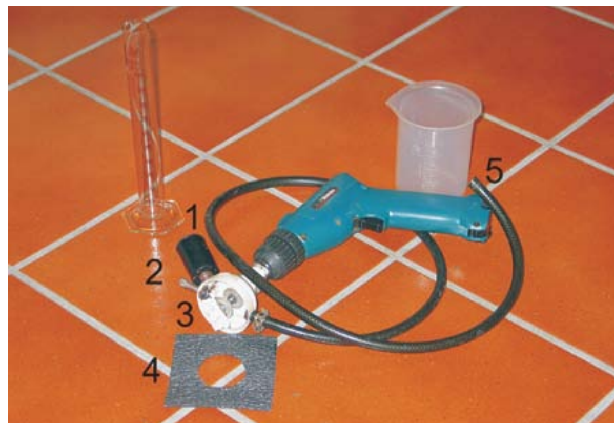
Fig. 6: A device for the chlorophyll a estimate per surface unit in cases where algae were strongly adhered to the surface. The device is composed of an inflow tube, into which distilled water is poured (1), a valve to prevent the formation of a vacuum (2), a brush fixed to a rotation axle and connected to a spring which enables a secure connection between the brush and the surface (3), and is rotated using a battery boring machine, packing (4), and an outflow tube to collect algae re-suspended in water (5).
