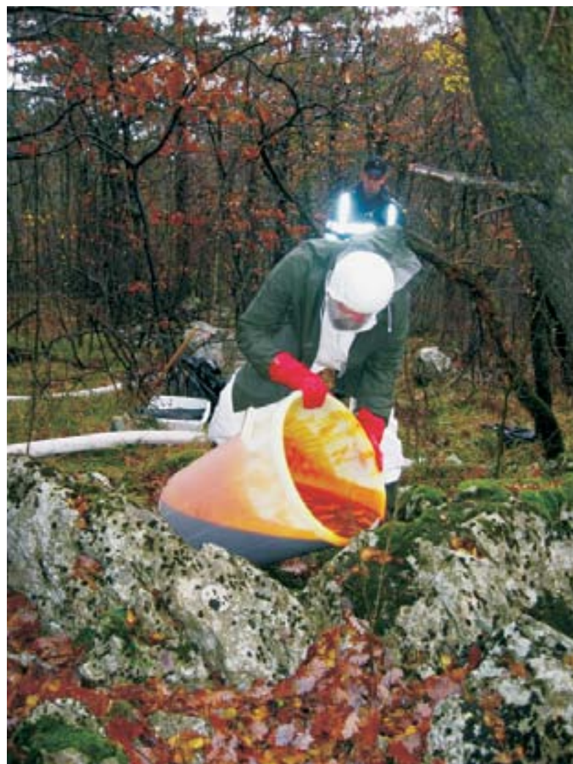
Fig. 3: Injection of Uranine on the surface by the Črnotiči quarry.
